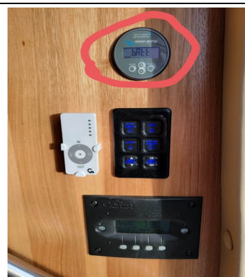
Battery monitor mounted on wall between pantry and door.
