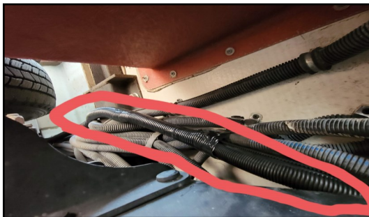
Typical shot of new wiring following and zip-tied to existing wiring.
