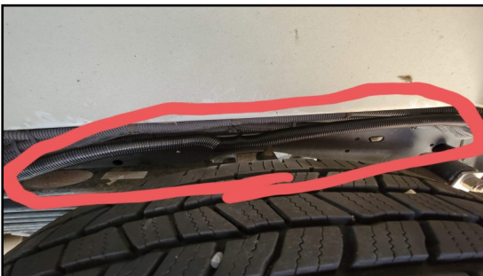
Wiring running through rear passenger side wheel well.
