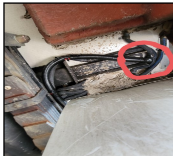
Circle shows the hole in the floor underneath the pantry.
