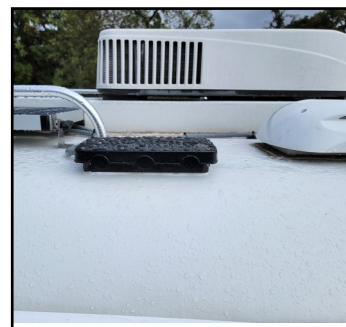
Combiner box mounted on roof and waterproof!
