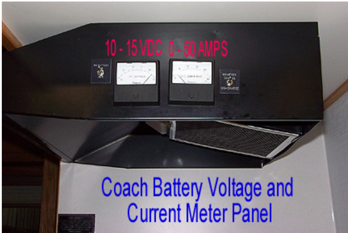
Figure 1 - 10-15 VDC Voltmeter and 0-50 AMP Ammeter Installed in Stove Hood
