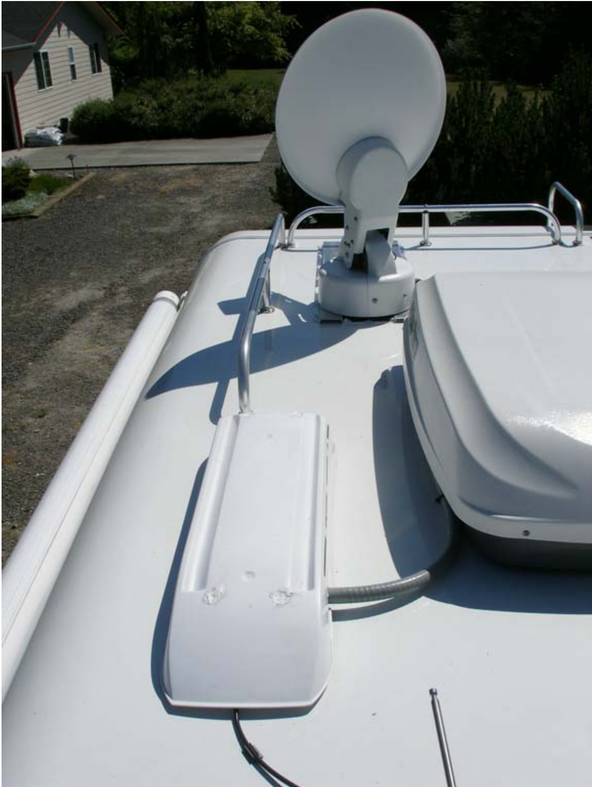
This shows how I attached the \frac{3}{4} " Flex to the air conditioner and attached to the Refrigerator vent.
