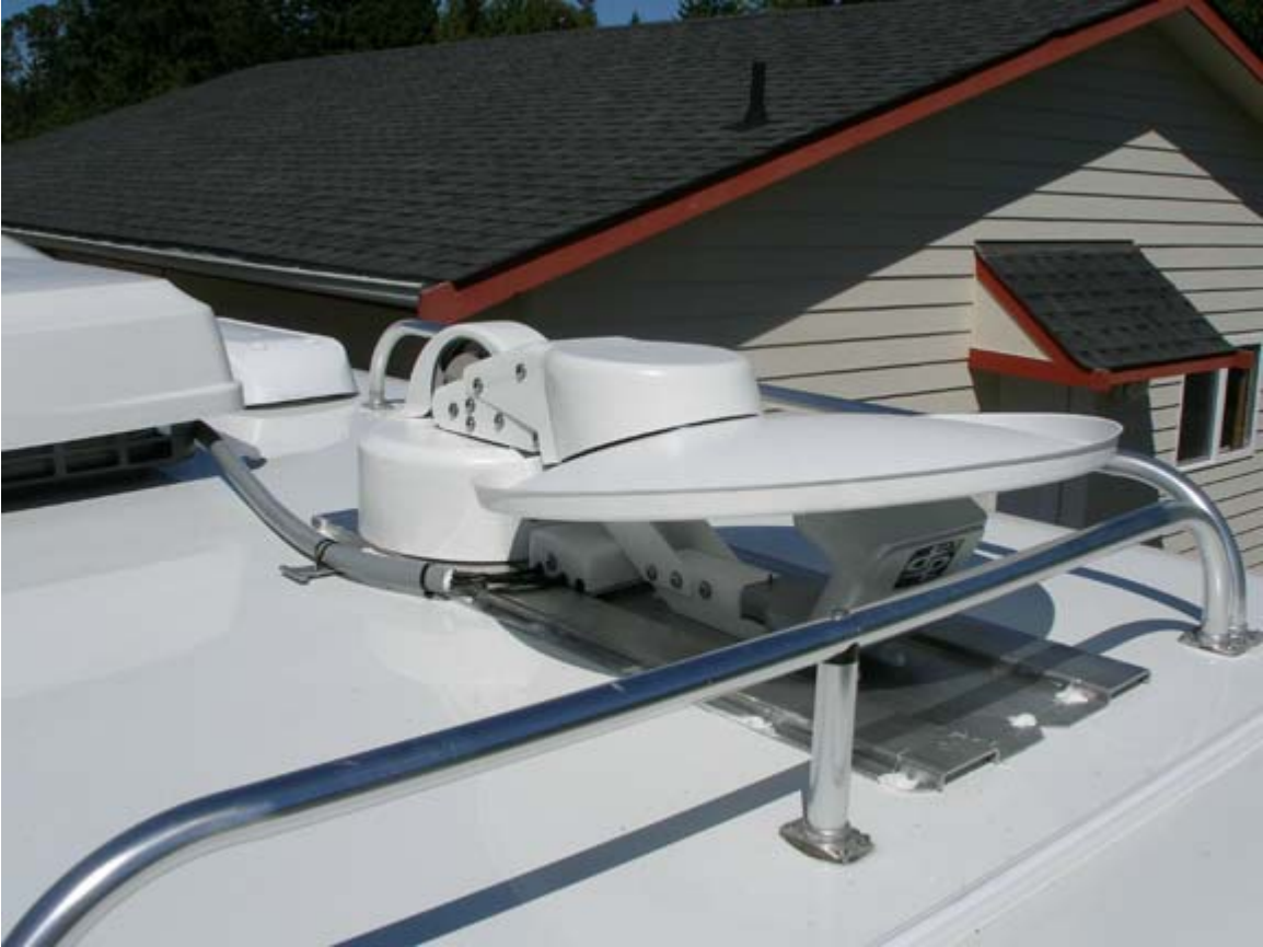
MotoSat MD500 stowed, it's only 10.5 inches high, will withstand 140MPH winds stowed and 60MPH deployed.
