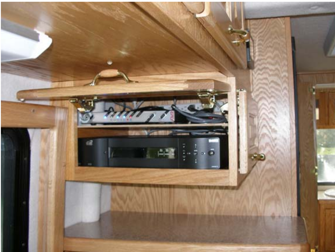
Nomad 2 controller on top, Dish 625 DVR Receiver on bottom. Not shown in photo is a layer of 3/8" closed cell foam under components for shock absorption.
