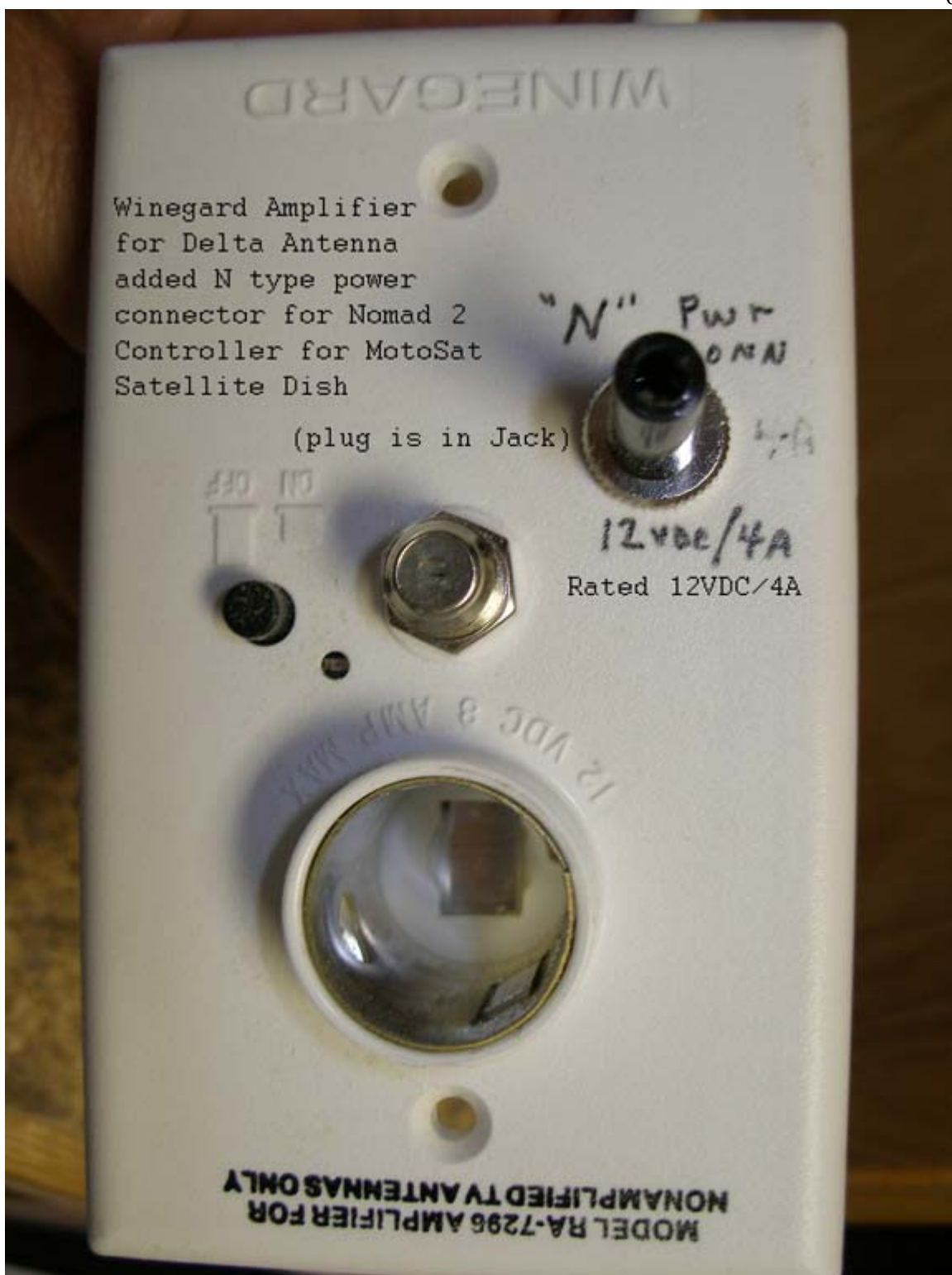
This is a close up of modified Winegard Amp cover
