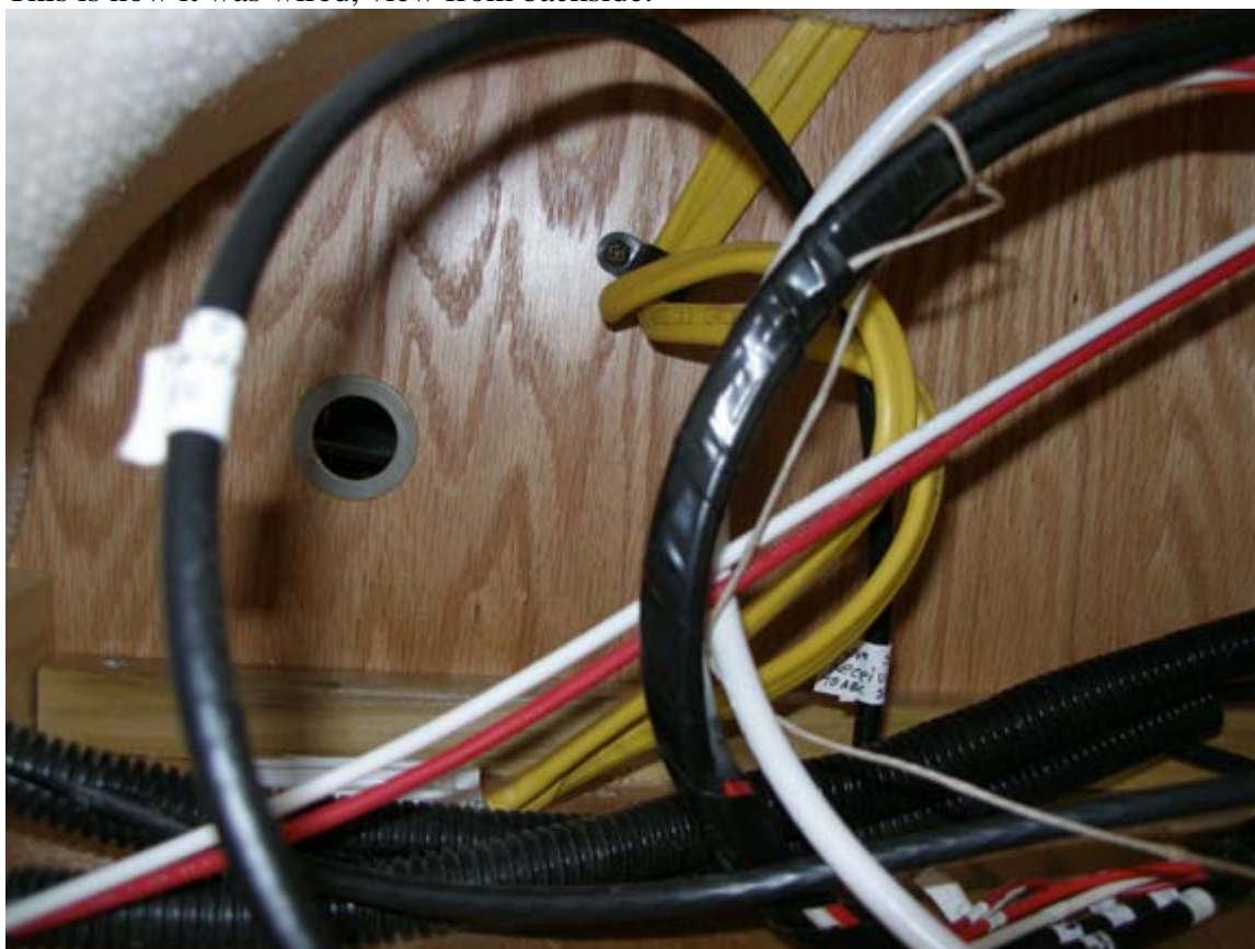
This is a picture of hole I drilled for wiring, this was used for some BF wiring and was convenient for placing my wiring. I also had some wiring here for a new Tank Monitor project I did but that's another project. The hole is actually behind the reefer.
