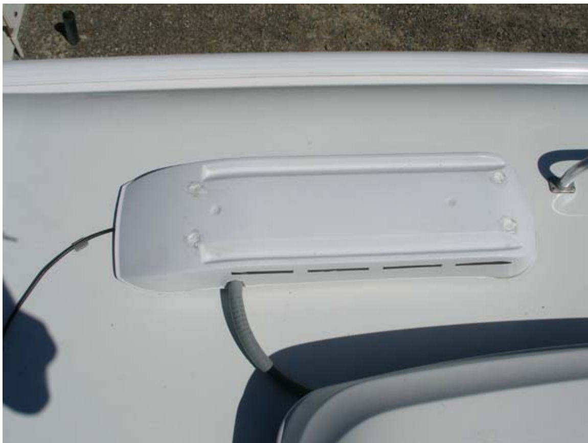
Close up view of 3/4" vinyl flex connected to reefer vent
