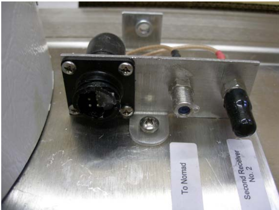
This is how the connectors are attached inside the small white box on base plate, note use of dielectric grease on connectors.
